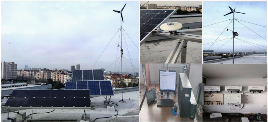
Figure 6. PV panels and measuring devices used in the experimental test.
