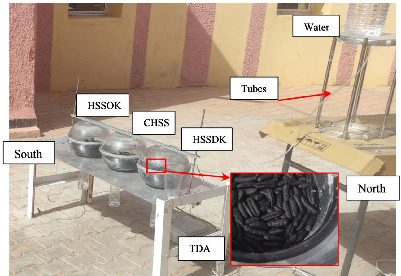
Fig. 1. The experimental setup of the proposed Hemispherical Solar Still (HSS) system.
